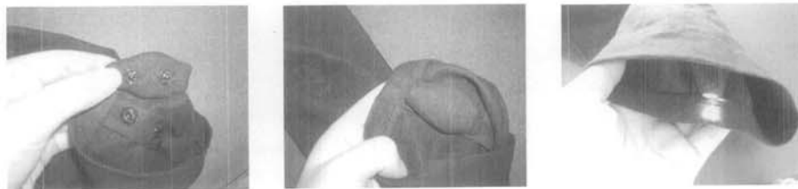
Fig. 10. Attachment of LED light using snap
