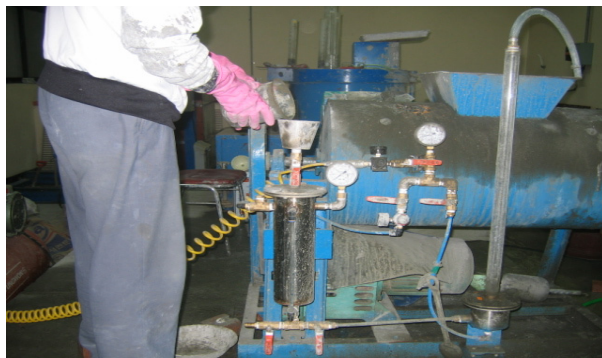
Fig. 2 Overview of putting foaming agent into a mixer
