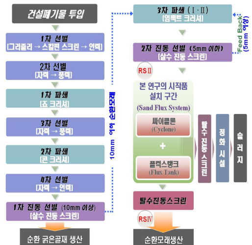
Fig. 2 Manufacturing process of recycled sand of the middle-treatment enterprise of construction waste
