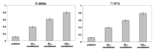
Fig. 3. Average surface roughness ( $R_a:\mu m$ ) of Ti alloys with various surface modifications.
