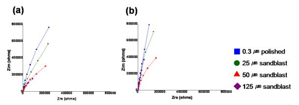
Fig. 7. Nyquist plot of MC3T3-E1 cell cultured Ti alloys after AC impedance test in 0.9% NaCl solution at  $36.5\pm1$ °C. (a) Ti-30Nb (b) Ti-30Ta.
