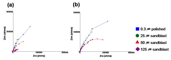
Fig. 6. Nyquist plot of non-cell cultured Ti alloys after AC impedance test in 0.9% NaCl solution at  $36.5\pm1$  °C. (a) Ti-30Nb (b) Ti-30Ta.
