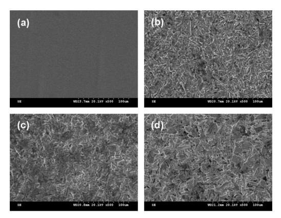
Fig. 2. SEM micrographs showing the non-cell cultured Ti-30Ta surface. (a) polished (b)  $25\mu$ m sandblasted (c)  $50\mu$ m sandblasted (d)  $125\mu$ m sandblasted.
