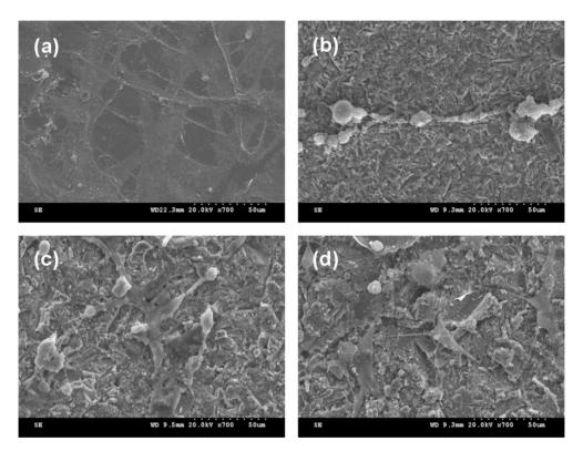
Fig. 4. SEM micrographs showing MC3T3-E1 cell cultured on Ti-30 Ta surface. (a) polished (b)  $25\mu$ m sandblasted (c)  $50\mu$ m sandblasted.
