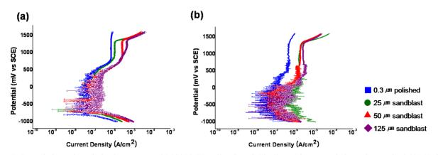
Fig. 5. Potentiodynamic polarization curves of MC3T3-E1 cell cultured Ti alloys after potentiodynamic test in 0.9% NaCl solution at  $36.5 \pm 1$ °C. (a) Ti-30Nb (b) Ti-30Ta.
