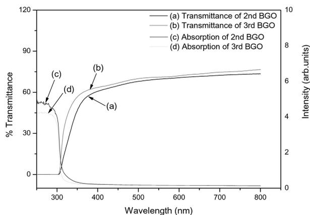
Fig. 1. Transmission and absorption spectra of the second and third grown BGO crystal.
