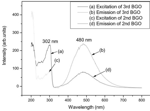
**Fig. 2.** Excitation and emission spectra of the second and third grown BGO crystal.
