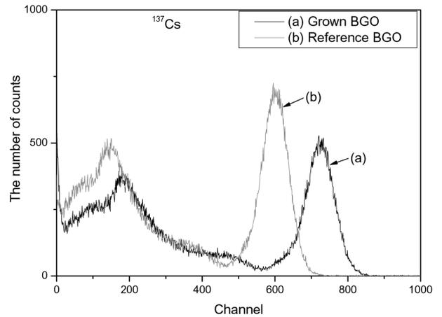
**Fig. 5.** Gamma ray spectrum of <sup>137</sup>Cs (662 keV).
