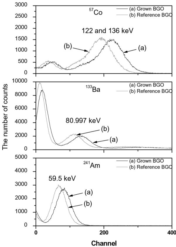
**Fig. 3.** Gamma ray spectra of <sup>241</sup>Am (59.5 keV), <sup>133</sup>Ba (81 keV) and <sup>57</sup>Co (122 and 136 keV).
