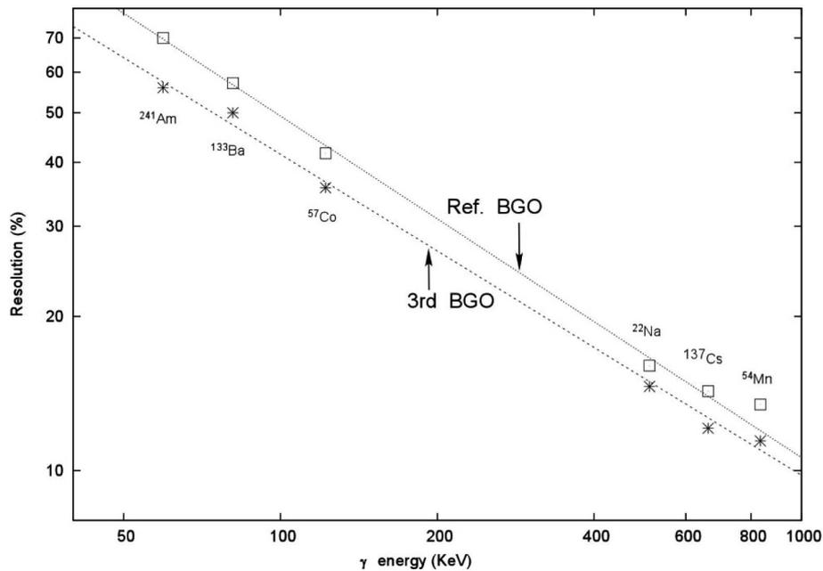
Fig. 7. Energy resolution of our third grown BGO ( $9.5 \times 9.5 \times 7.5 \text{ mm}^3$ ) and reference BGO ( $10 \times 10 \times 10 \text{ mm}^3$ ) as a function of gamma-ray energy.
