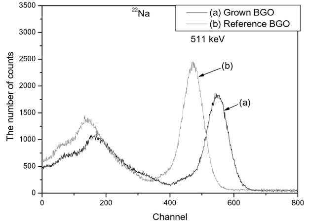
**Fig. 4.** Gamma ray spectrum of <sup>22</sup>Na (511 keV).
