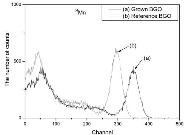
**Fig. 6.** Gamma ray spectrum of <sup>54</sup>Mn (834 keV).
