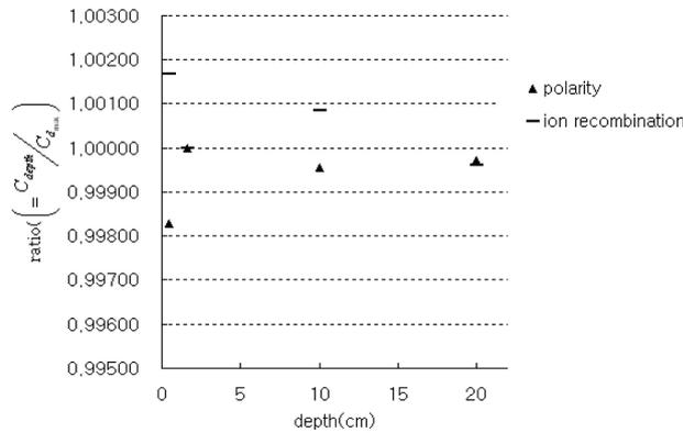
**Fig. 3.** Polarity and ion recombination effects of a semiflex chamber (PTW 31010<sup>TM</sup>, SN 1551) with depth in water for the photon-6 MV beam. The correction factors on the y-axis are normalized to the factor at the  $d_{max}$ , the depth of the maximum dose because the PDDs are the quantities normalized to the maximum dose depth  $d_{max}$ .
