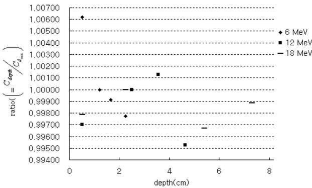
**Fig. 5.** Ion recombination effects of a semiflex chamber (PTW 31010™, SN 1551) with depth in water for the electron-6 MeV, 12 MeV, and 18 MeV beams. The correction factors on the y-axis are normalized to the factor at the  $d_{max}$ , the depth of the maximum dose because the PDDs are the quantities normalized to the maximum dose depth  $d_{max}$ .
