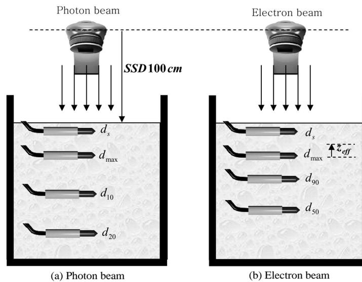
**Fig. 2.** Schematic drawing of the setup for experimental measurements. For the (a) photon beam the 4 depths of  $d_s$ ,  $d_{max}$ ,  $d_{10}$ , and  $d_{20}$  were chosen, while for the (b) electron beam the 4 depths of  $d_s$ ,  $d_{max}$ ,  $d_{90}$ , and  $d_{50}$  were used. The  $0.5 r_{cyl}$  (the inner radius of the chamber) were used as the effective point of measurements  $z_{eff}$  in the electron beam and the **100 cm** was set up as the source to the surface distance **SSD**.
