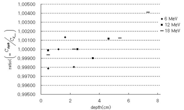
**Fig. 4.** Polarity effects of a semiflex chamber (PTW 31010<sup>TM</sup>, SN 1551) with depth in water for the electron-6 MeV, 12 MeV, and 18 MeV beams. The correction factors on the y-axis are normalized to the factor at the  $d_{max}$ , the depth of the maximum dose because the PDDs are the quantities normalized to the maximum dose depth  $d_{max}$ .
