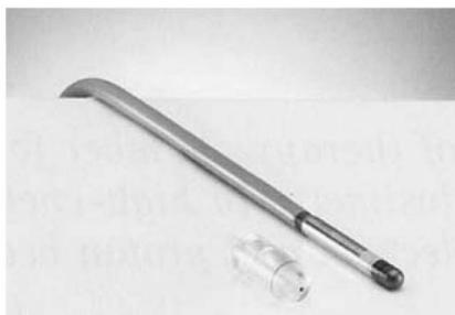
(a) Semiflex ionization chamber
