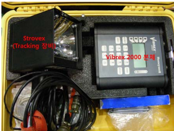
Fig. 7 Blade Tracking & Balancing Kit
