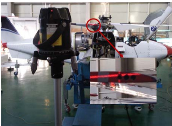
Fig. 4 Rotor Rotating Plane Adjustment
