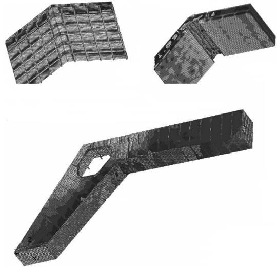
Fig. 9 Equivalent stress distribution at membrane, R-PUF and hull structure
