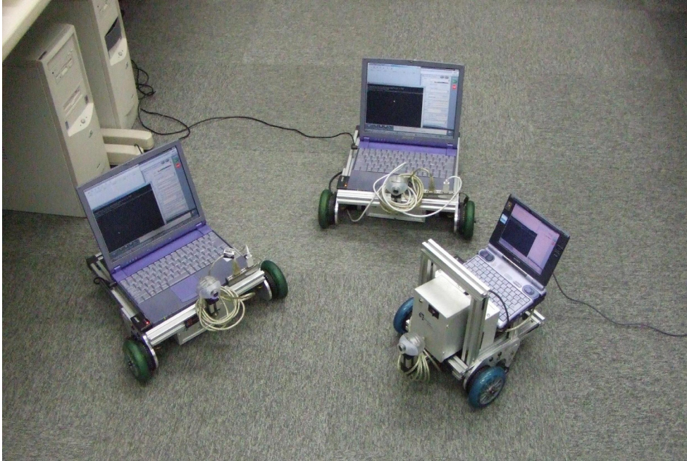
Figure 11. A team of mobile robots work under control of mobile agents.
