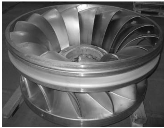
Fig. 2 Runner A, before experimental setup
