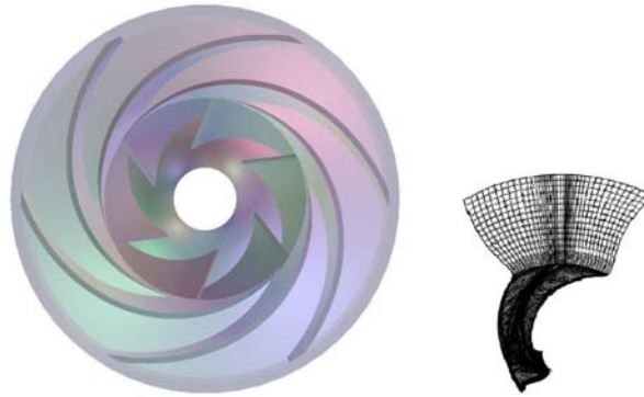
Fig. 3 3D geometry and grid system of the impeller (3)
