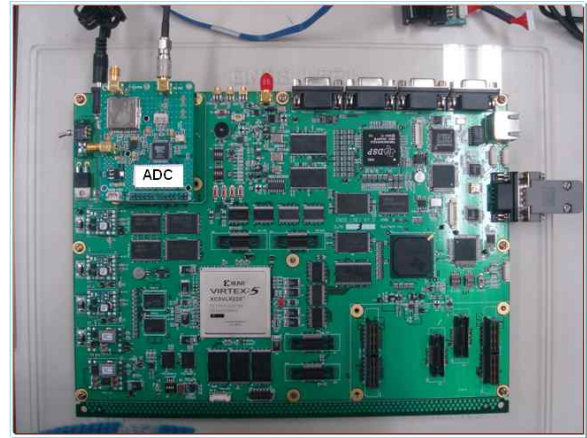
Fig. 8. Signal Processing Configuration Based on FPGA.
