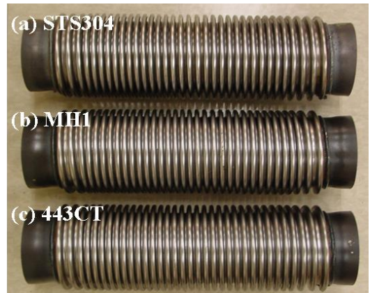
Fig. 5 Multi-layer bellows manufactured in the present study by roll forming with different materials
