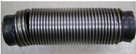
Fig. 7 Fractured 443CT multi-layer bellows after fatigue test
