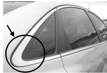
Fig. 1 Typical surround molding part
