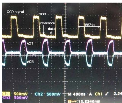
Fig. 13. CCD signal and the differential output of VGA with the gain of 36 dB
