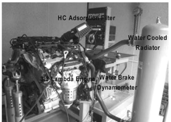
Fig. 5 Photo of engine test bench
