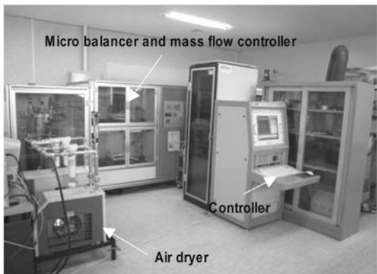
Fig. 4 Photo of BWC experimental set-up
