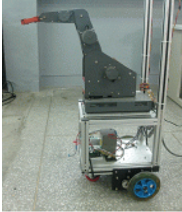
Fig. 1 Structure of M2 Platform
