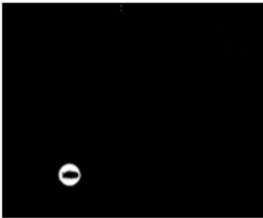
Fig. 3.6 Marker Detection using Binarization
