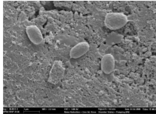
Fig. 1. A SEM image of Bacillus subtilis ATCC 6633 attached to Al-Fe bimetallic oxide-coated sand (Bar = 1 μm).
