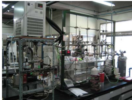
Fig. 1. Image of volumetric adsorption system for PA adsorption on ACFs.
