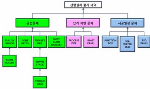
Fig. 6 Pre-outfitting fault tree
