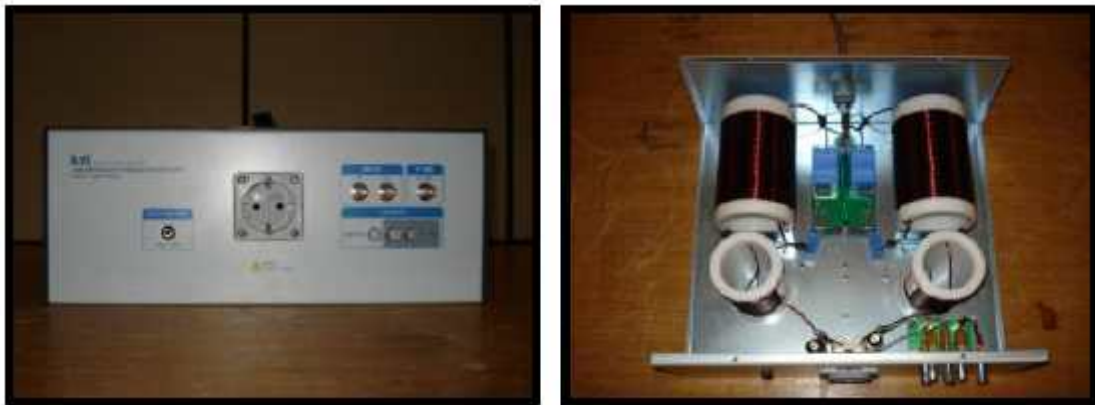
<Figure 3> LISN made for the test
