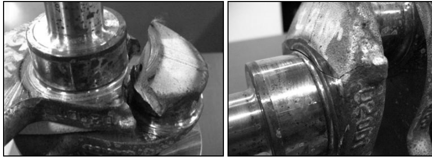
Figure 3.2. Failure mode during bending test.
