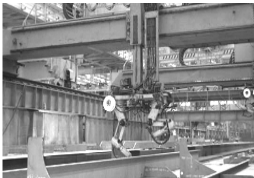
Fig. 1 Robot welding shop for subassembly
