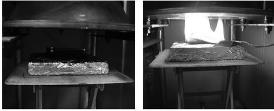
(a) Glowing mode ignition (b) Flaming mode ignition
