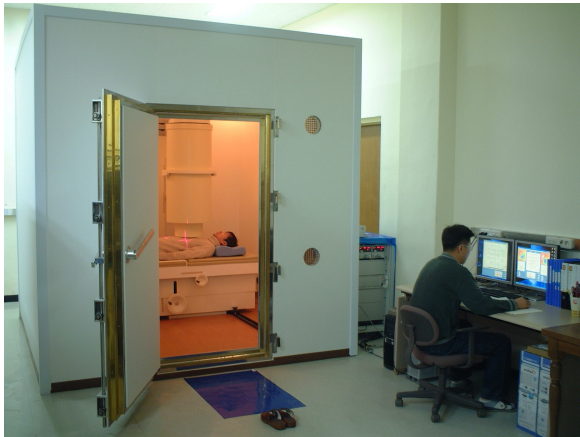
Fig. 3. Photograph of magnetically shielded room(MSR) and 61 channel SQUID system for measuring biomagnetism.
