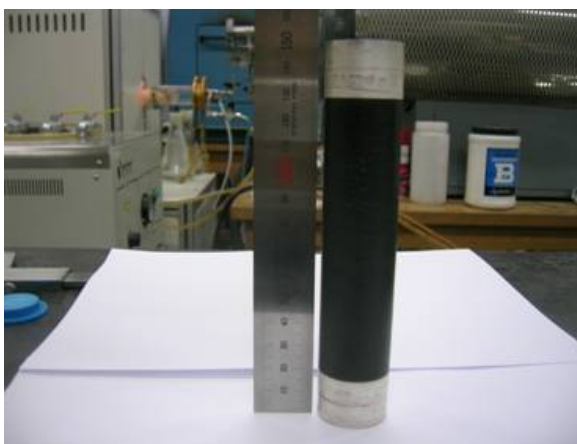
Fig. 2. BSCCO tube fabricated by centrifugal melting process. (30 Φ×150 h×4 t)
