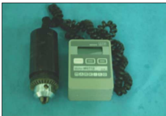
Fig. 8. The photograph of torque gauge; removal torque was measured with MGT50 torque gauge.
