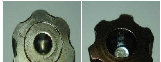
(c) one projection on punch (d) change of punch shape & Friction Factor
