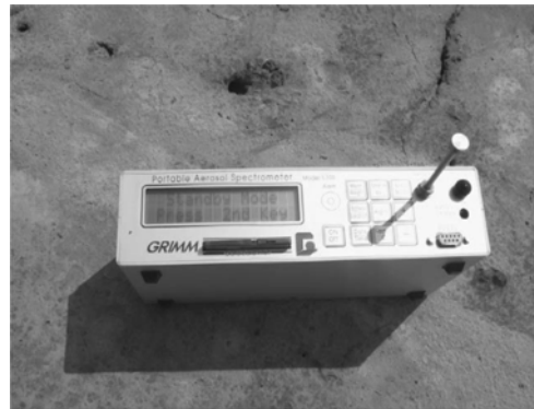
Fig. 2 Dust spectrometer on the reclaimed land in Gim-je area
