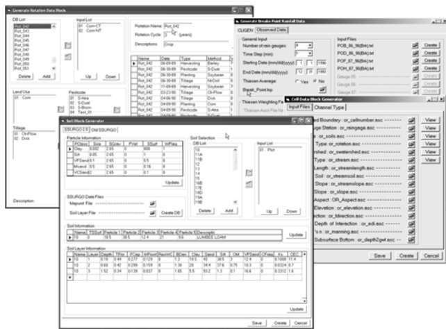
Fig. 7 Interface windows provided by the developed interface for generating rainfall input and soil, cell, and rotation data blocks
