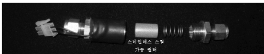
Fig. 7. Swagelok® Inline Filter Holder with 7 \mu m Sintered Stainless Steel Filter.
