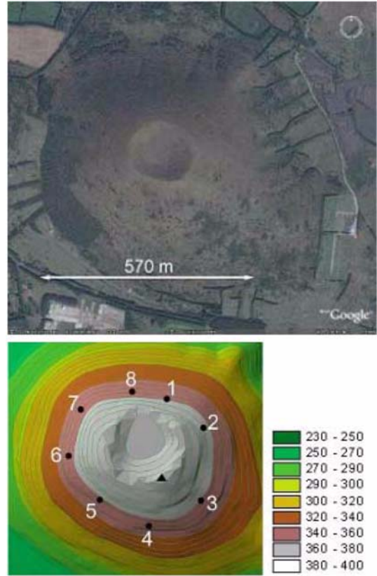
Fig. 1. A satellite image of the parasitic volcano (top) and locations of 8 solar irradiance measurement points (circle) and 1 reference solar radiation site (triangle) on the elevation map of the volcano (bottom).
