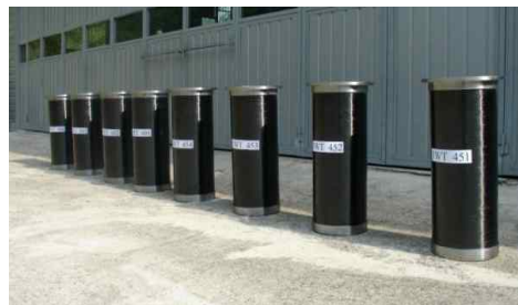
Fig. 2. Composite cylinders before test
