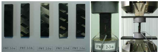
Fig. 4. Effective modulus test specimens and set-up
