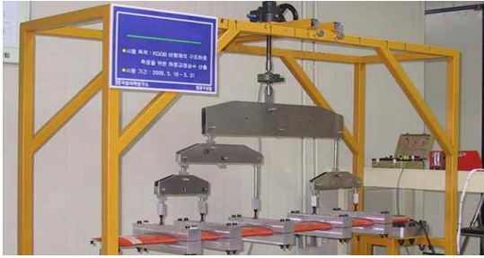
Fig. 3. Ground static test of glider's wing
