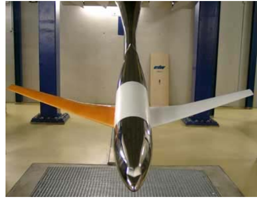
Fig. 2. Wind tunnel model for DLR-F4 configuration
