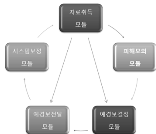
Fig. 2. Warning System Processes.
