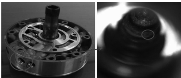
(a) Inner shrinkage of Machining hole
