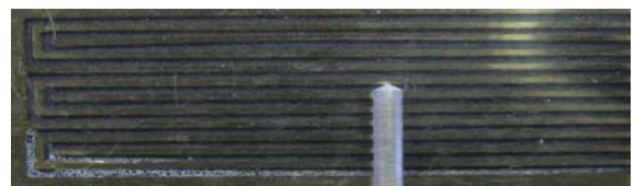
Fig. 13 Cathode channel flooding at left bottom triangular zone @V cell =0.5V, I ave =0.91A/cm 2
