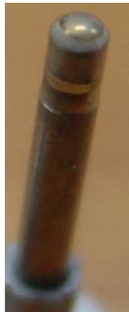
Fig. 8 Injector needle after durability test
