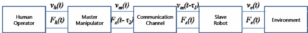
Fig. 9 2-port network representation of teleoperation system
