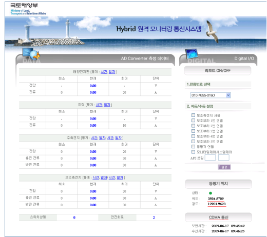
Figure 9: The monitoring program of the CDMA tele-controlling system
