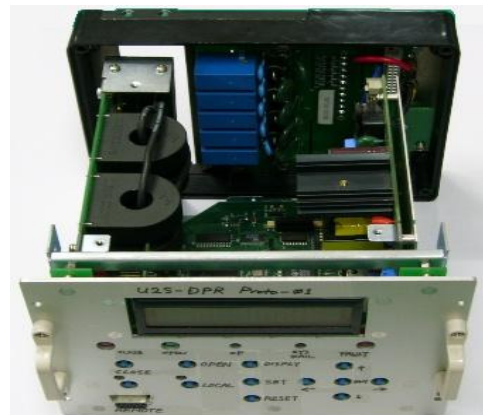
Figure 7: Hardware of digital protective relay
