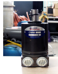
Figure 3: Photo of oil pressure operating motor
