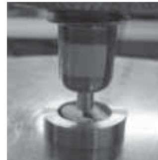
Fig. 2. Contact diameter 1.2mm in central part and road to head speed 0.5mm/min
