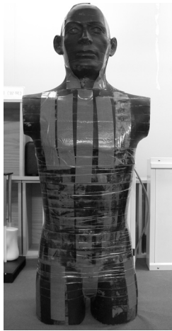
Figure 2. Rando man phantom
