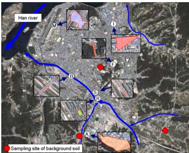
Fig. 1. Investigation point and drainage area of dredged soil classified by drainage type.
