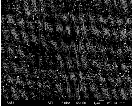
Fig. 4. The misoriented YBCO grain in film fired at 780°C for 2 h.
