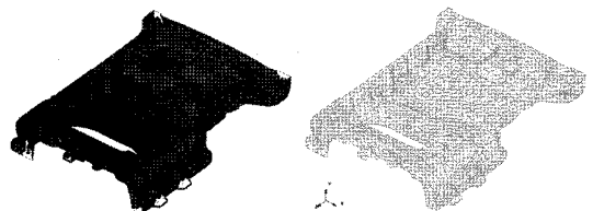
Fig. 3 Shape and finite element model of oil pan upper
