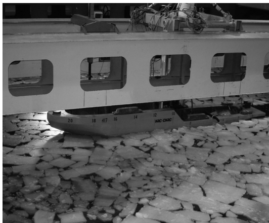
Fig. 2 The profile of self-propulsion test with refrigerated ice
