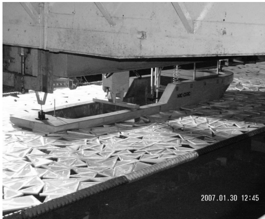
Fig. 1 The profile of self-propulsion test with synthetic ice
